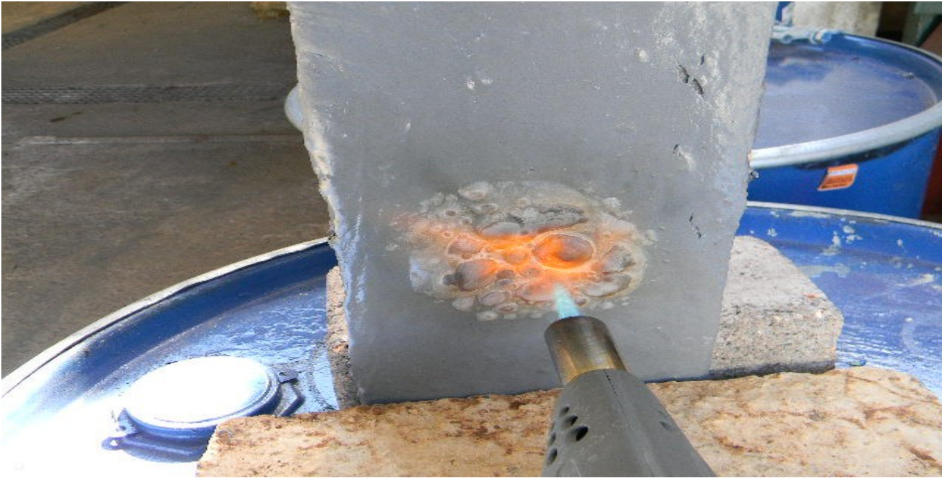
A butane gas flame was focused on the coating for 2 hours
